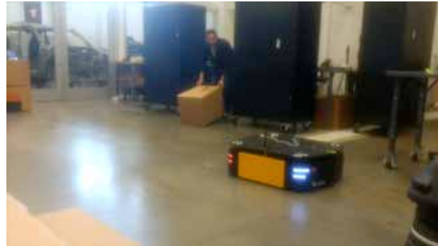
Ridgeback dynamic obstacle avoidance (slow moving) using teb_local_planner
