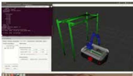
Simulation development using MoveIt! in ROS
