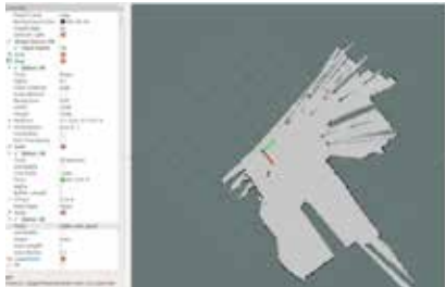
SLAM using offline ROS processing (replayed from LiDAR rosbags of manually driven YMR12)
