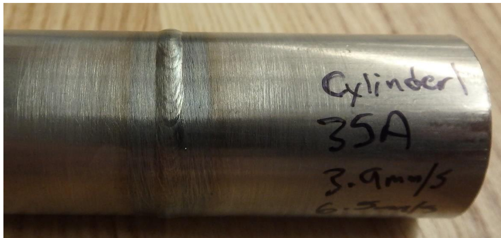
Successful welds on tube sections with variable gap+mismatch
