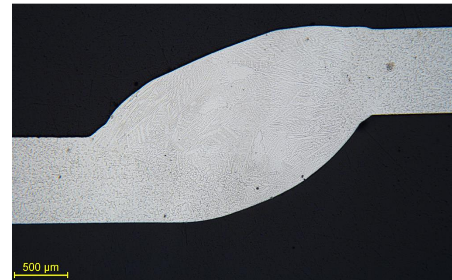
Challenge coupon: 0.0" gap, 0.032" mismatch Successful weld
