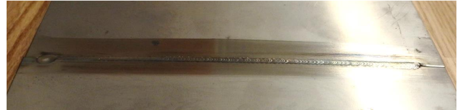
Variable mismatch with changing weave plane 0.015" gap, 0.015" → 0.0" → -0.015" mismatch,
