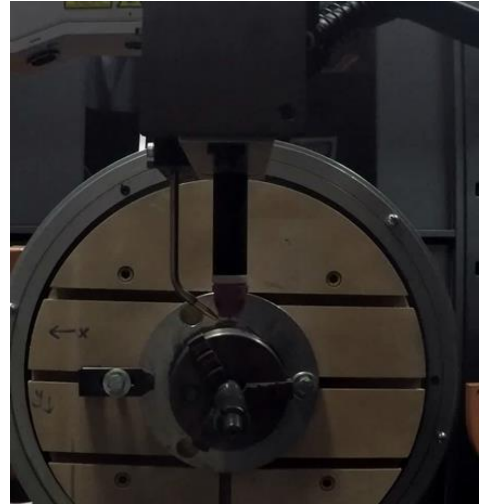
Turntable with coordinated motion, maintains prescribed travel speed and weave on non-flat parts
